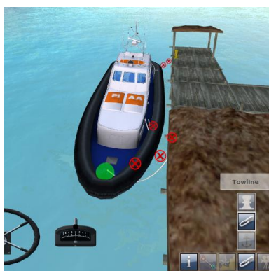
Figure 8b. Towline connection points are visible as green spheres.
