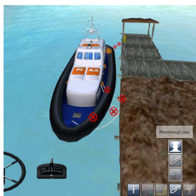
Figure 8a. Mooring lines. Connection points are shown as orange spheres.
