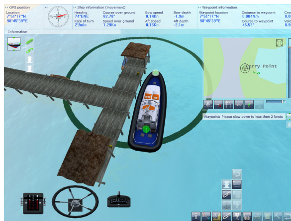
Image 19. Next waypoints are to moor the ship again at its original location. Sail to the green circle, click on the mooring icon. Then click on an orange dot on the ship and next on the orange dot on the mooring boulder. A mooring line is created and the waypoint is achieved.
