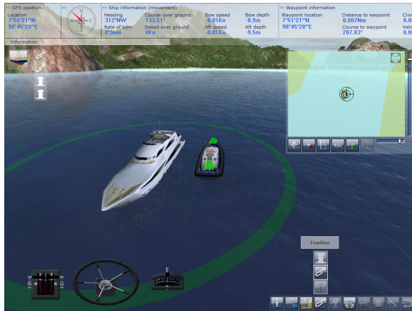
Image 11. Click again on the Moorage icon at the bottom, then on the Towline icon. Green dots will appear on the front and back of the ship, indicating the connection points. Now click on one of the green dots, then on the orange dot on the yacht's front. Now your towing rope is connected.
