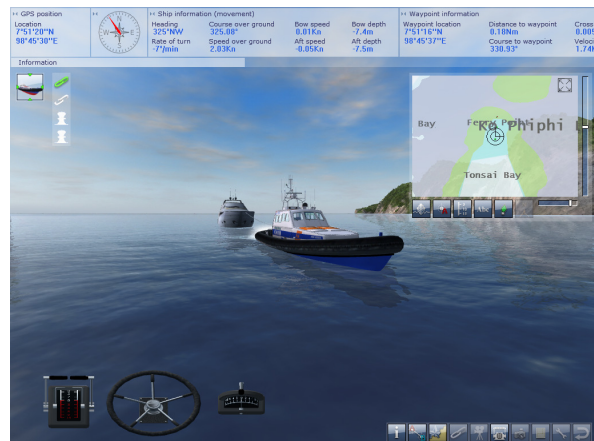
Image 14. Keep track of the chart. The little green arrow on the edge of the circle indicates the direction you need to go to the next waypoint.
