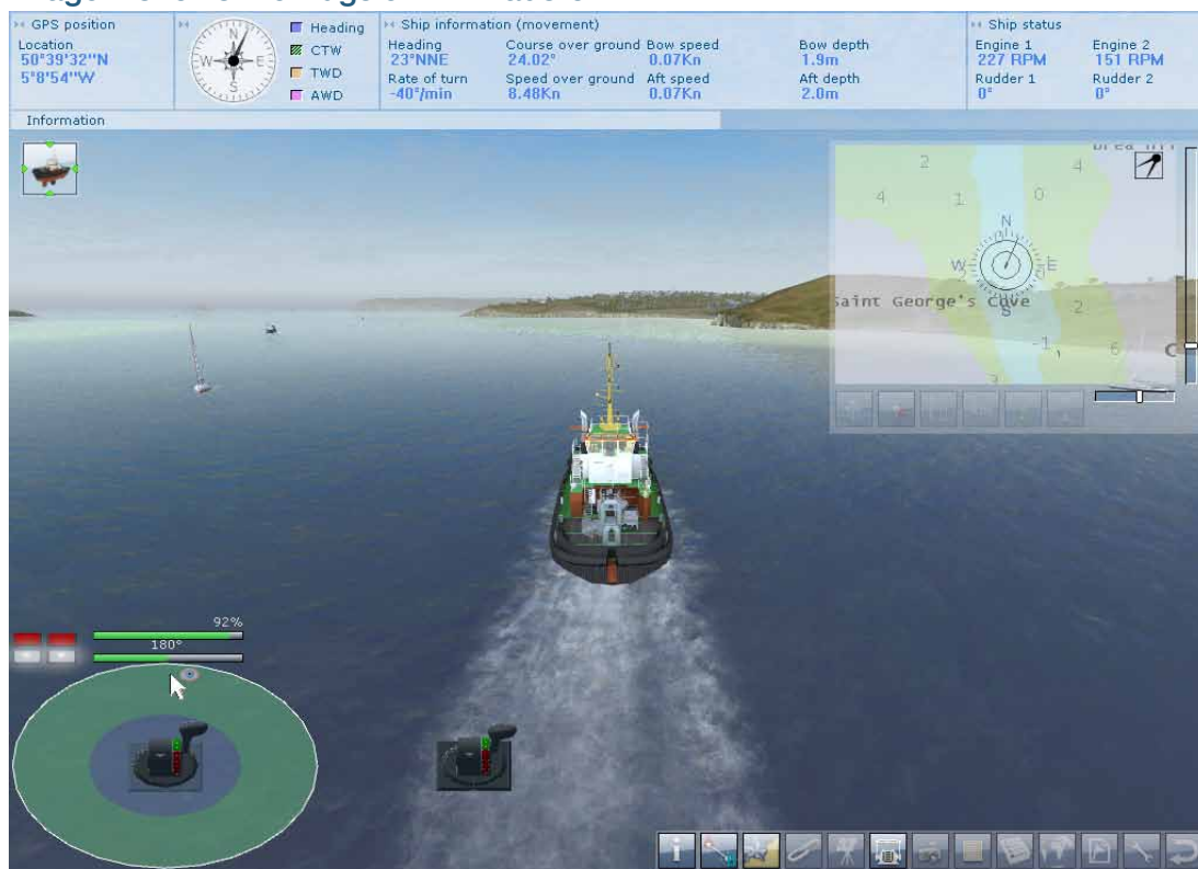
Image 2. Bugsier 2 in Padstow. This thruster cannot be set in the reverse position. Instead, to reverse, you need to rotate the thruster 180 degrees, by dragging the mouse left/right in the blue circle.
