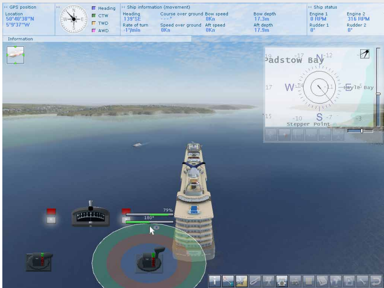
Image 1. Controlling the cruise ship with azimuth thrusters. Moving the cursor over the thruster control brings up several circles. The green circle is used for setting the forward thrust, the red circle for the reverse thrust, and the blue inner circle is used for setting the thruster rotation. You set the forward thrust by click-dragging the cursor up and down in the green circle. Similarly, you set the reverse thrust by click-dragging the cursor in the red circle. Lastly, you set the direction of the azimuth thruster by click-dragging the mouse left and right in the blue circle. This is best done in the bottom half of the blue circle.
