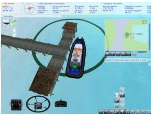
Image 19. Next waypoints are to moor the ship again at its original location. Sail to the green circle, click on the mooring icon. Then click on an orange dot on the ship and next on the orange dot on the mooring
